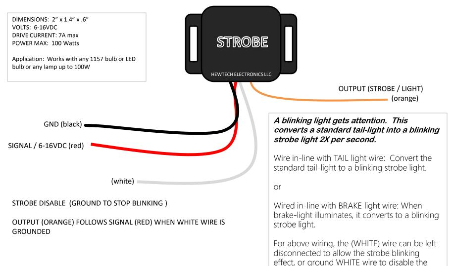
blinking and convert the output back to original lighting function (no blinking)
