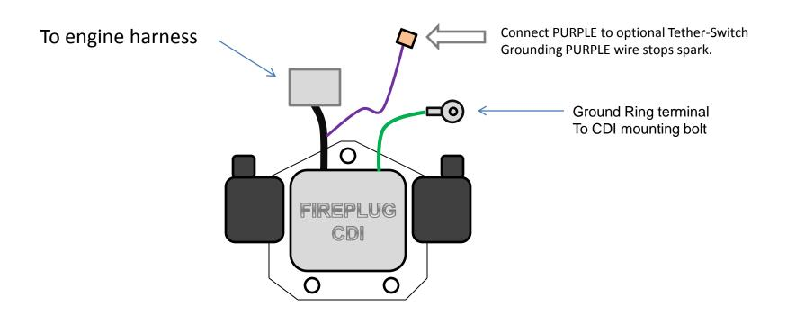
If not using a 2-wire Tether or Kill-Switch, PURPLE wire not connected Original 3-wire kill-switch requires no additional wiring.
